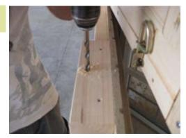
Use 3/16" bit and drill hole in bottom of door as shown.
